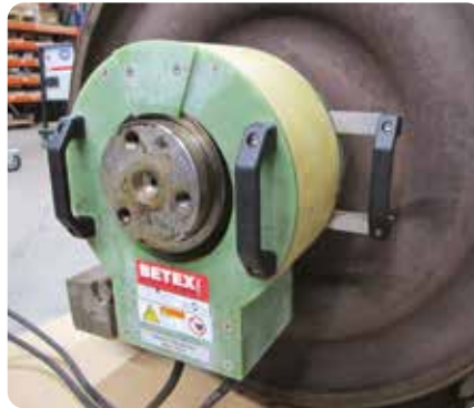
Heating bearing rings for dismounting
