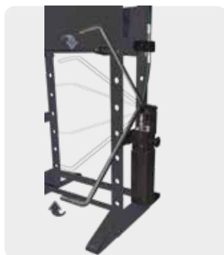
Hand and foot pedal for double operation
