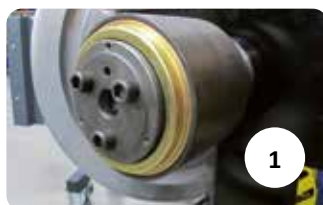
Step-by-step dismounting of TBU / SP / TAROL bearing sets
