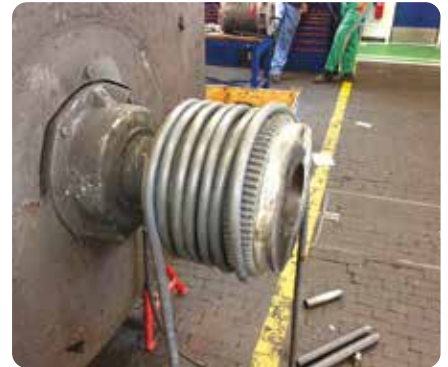
Heating a coupling for dismounting
